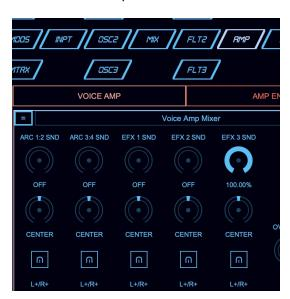
In the Global Sections (EFX, etc), there are two stereo busses dedicated to ARC (Audio rate control), these can be used as dual stereo, or as 4 single busses, or whatever combination you prefer, as it is up to you how you want to use them. The VOICE AMP section allows you to put Voice level signals on the Global ARC busses, and in the Main Pre Mixer, you can also choose the Main Feedback, Audio/Side-Chain inputs to be Audio Rate modulation bus sources.
