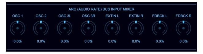
Not all of the Filters currently support the ARC bus, but a lot of them do, along with other types of filter processors, like the Wavefolder, which can use the ARC bus signal to achieve audio rate Drive Modulation. When you see the ARC parameters in a Filter, you will have control of the bi-polar amount of curve (re-shaping) of the ARC bus to use as an audio-rate modulator for a specific function in that filter.
